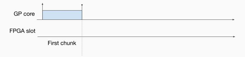
• After a **contention phase** (shared resources (area) and reconfiguration interface) the **HW-task** is **configured** on the FPGA
